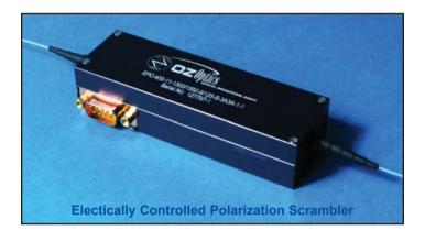
The polarization controller is available in either a three or four channel configuration. The three channel system is ideal for polarization scrambling applications such as for polarization averaging or PDL measurements. The added redundancy of the four channel version opens the way to continuous polarization control, without having to occasionally reset the device when a controller reaches its limit.
